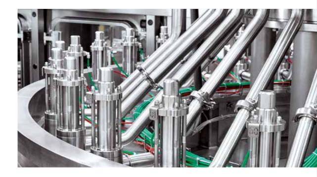
Non-contact volumetric filling with weighing cell, i.e. there is no contact between the bottle and filling valve during entire fill process, thus protecting the filled product against scraps dripping from worn seals.
