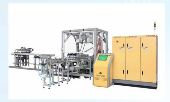
After this line is put into the production, it can assemble four frames simultaneously, help to save 6-8 workers, and enhance the production efficiency by 30%.
